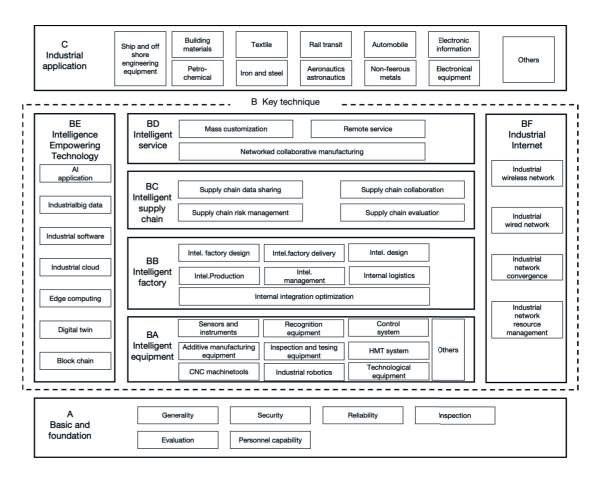
Figure 5: Structural Diagram of Intelligent Manufacturing Standard [28]
